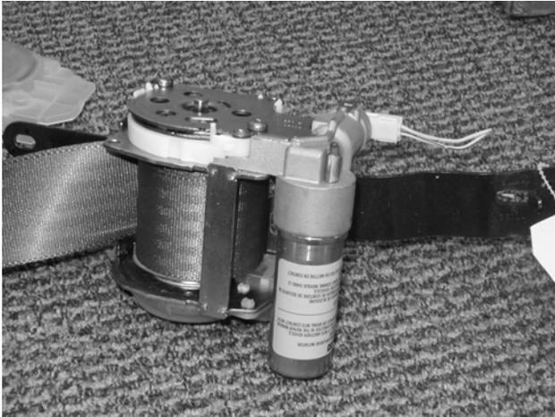
Figure 2. Shoulder Belt Retractor Pretensioner
